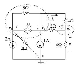
First, choose the reference point and number the node voltages  $v_1$ ,  $v_2$  and  $v_3$ .
